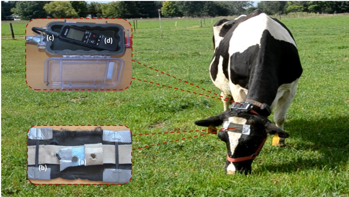
Figure 1. Recording system used to record the acoustic signals composed of inward and outward facing microphones (a). Wired microphones were covered by an elastic headband (b) and plugged (c) into a recorder housed inside a weather proof case attached to the top side of a halter neck strap (d).
