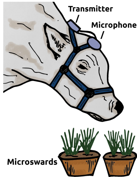
Figure 2: Microphone was located facing inwards on the forehead of the cow and the transmitter was placed on the neck. The cow is grazing microswards.
