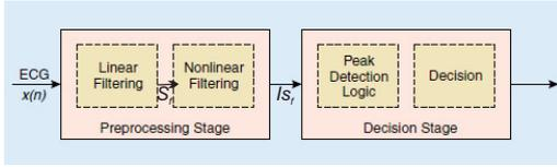
Fig. 1: Typical structure of a classical QRS detector [6].
