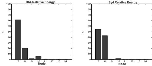
Fig. 4: FWPT relative energy of the 8 terminal nodes of a QRS (where 7 corresponds to node (3,0), 8 to (3,1), etc.). In the left panel the result is obtained by Daubechies 4 mother wavelet and in the right panel with Symmlets 4.
