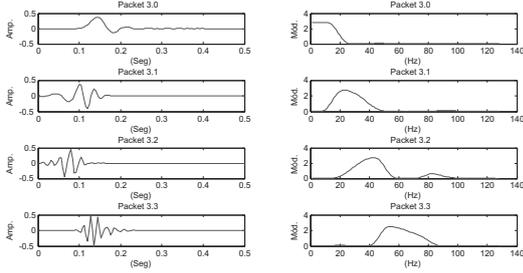
Fig. 3: Different scale 3 atoms of Daubechies mother wavelet with 5 zero null moments with there spectrums. Sampling frequency of 250 Hz.
