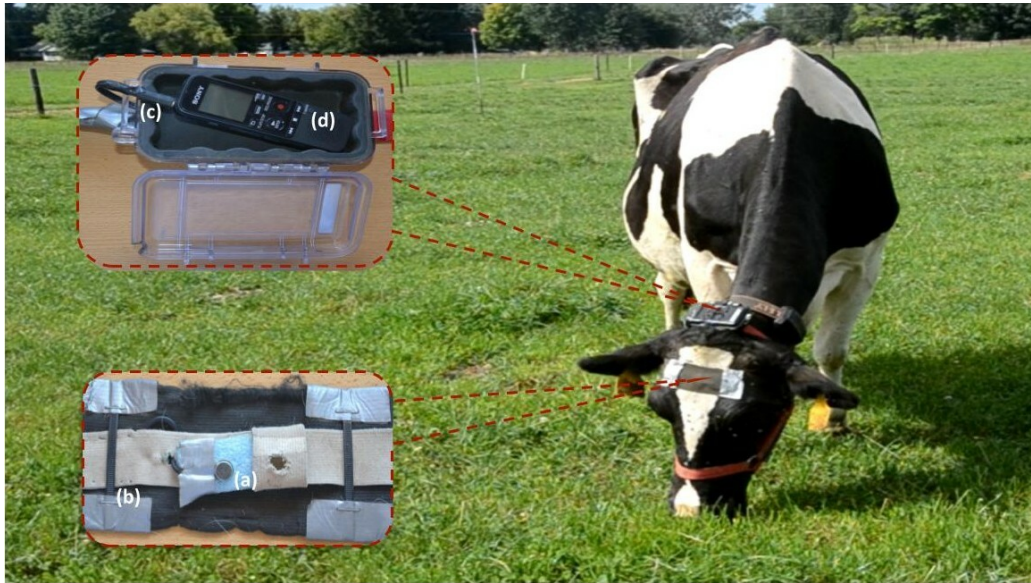
Figure 3: Recording system used to record the acoustic signals composed of microphones (a) that are covered by rubber foam and an elastic headband (b), which are wired and plugged (c) to a digital recorder placed inside a waterproof case (d) attached to a neck halter. Figure extracted from Martinez-Rau et al. (2023b)
